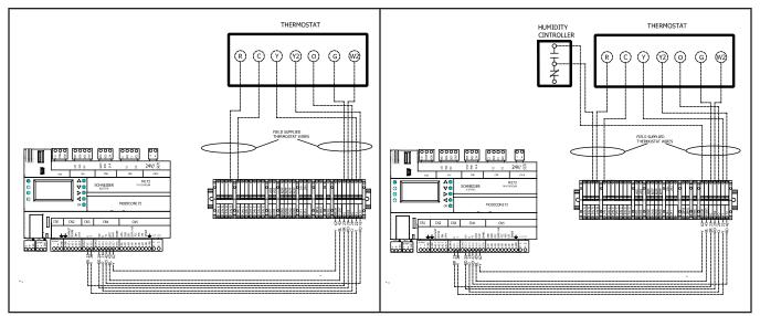
Figure 6a. Remote Wall Mounted Thermostat Wiring Detail
