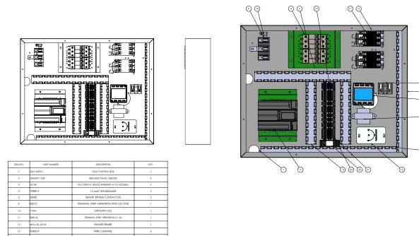
Figure 9b. Typical Control Center Layout for 3-Phase Scholar 2.0
