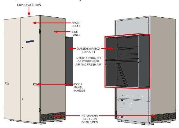
Figure 1. General External Component Identification and Access to Scholar 2.0
