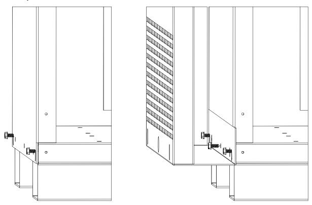
With a firm grip on the edge of the panel, slightly swing the panel away from the unit while you lift and pull the panel away from the guide flange.
