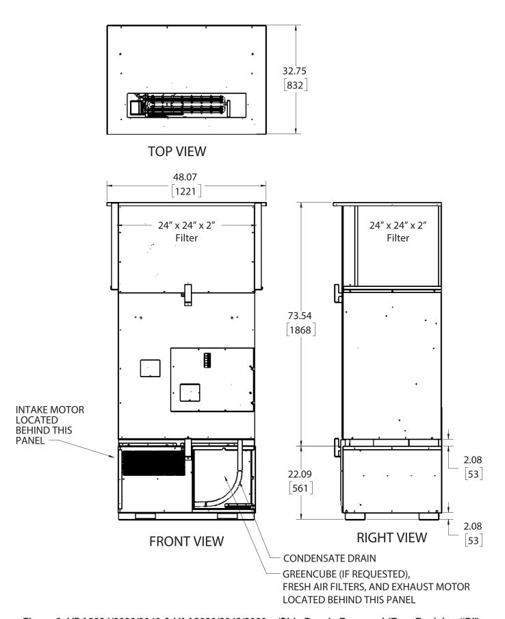
Figure 3. VDA2024/2036/2040 & VAA2030/2048/2060 w/Side Panels Removed (Eng. Revision "B")
