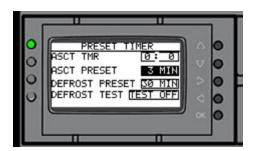
The Anti short cycle protects the system compressor from short cycling due to excessive on and off, this can happen when there is a fault or someone turning the system off and on for troubleshooting purpose etc. This timer starts timing when the compressor turns off and prohibits it from running again until the time period as elapsed.
