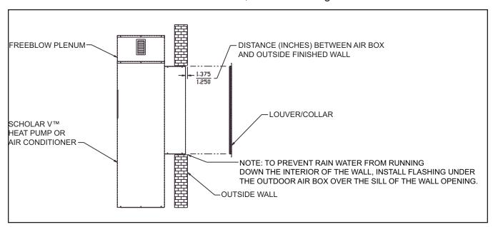
Figure 1. Dimension between Scholar 2.0 Air Box and Finished Outside Wall for Outdoor Louver/Collar Assembly Installation.
