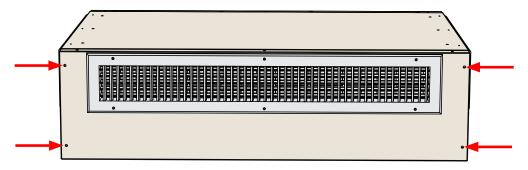
2. On the top panel of the Scholar 2.0 unit, locate the 6 holes that correspond with the six mounting holes in the plenum.
