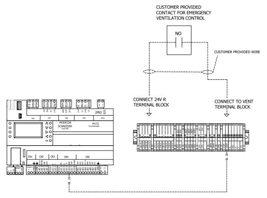
FOR EMERGENCY VENTILATION CONTROL, END USER SHOULD PROVIDE NORMALLY OPEN CONTACT AND CONNECT TO "24V R" AND VENT INPUT TERMINAL BLOCK, AS SHOWN, WHEN CONTACT IS CLOSED EMERGENCY VENTILATION OPERATION IS ACTIVE.
