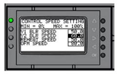
Use the right or left arrow key to navigate to the "Control Speed Settings" screen.
