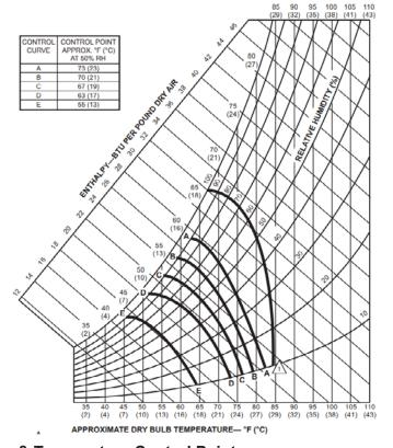
Figure 2. Enthalpy Sensor & Temperature Control Points
