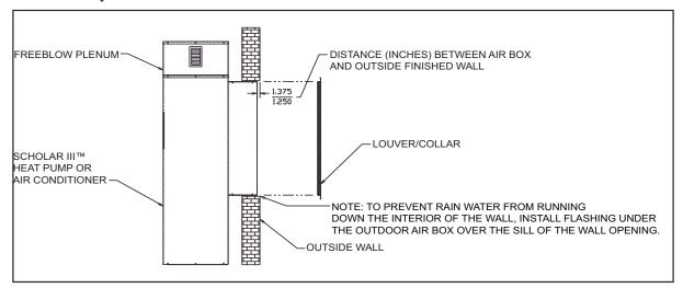
Figure 5. Dimension Between Scholar 2.0 Heat Pump or Air Conditioner Air Box and Finished Outside Wall for Outdoor Louver/Collar Assembly Installation
