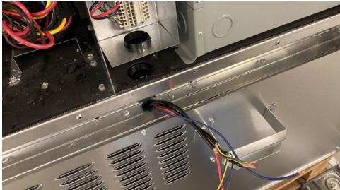
F. Disconnect the condensate drain tube.
