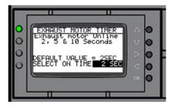
The exhaust motor timer is to adjust the time it takes to Vent (ventilation) output to energized which will then send 24VAC to the exhaust motor relay coil. The default time is 2 seconds, which can be changed from 2, 5 and 10 seconds.
