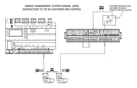
FOR CUSTOMER EMS CONTROL, END USER SHOULD PROVIDE ADDITIONAL WIRES GOING TO AND FROM THE END USER NORMALLY CLOSED CONTACT.
